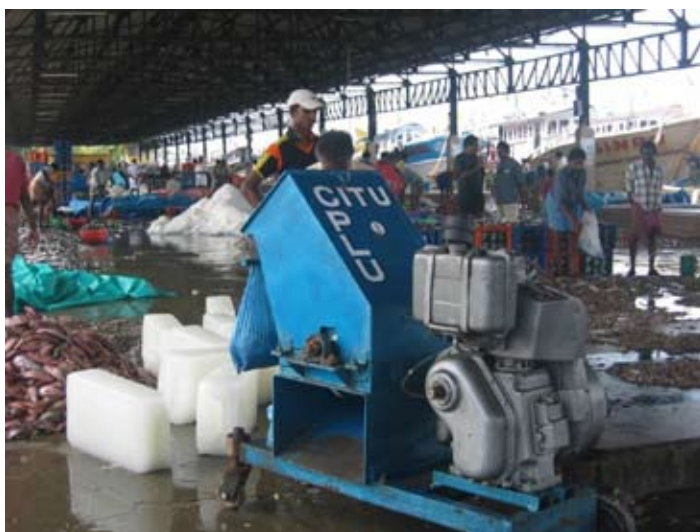
Ice crushing machine in operation at Marine fishing harbour at Cochin
