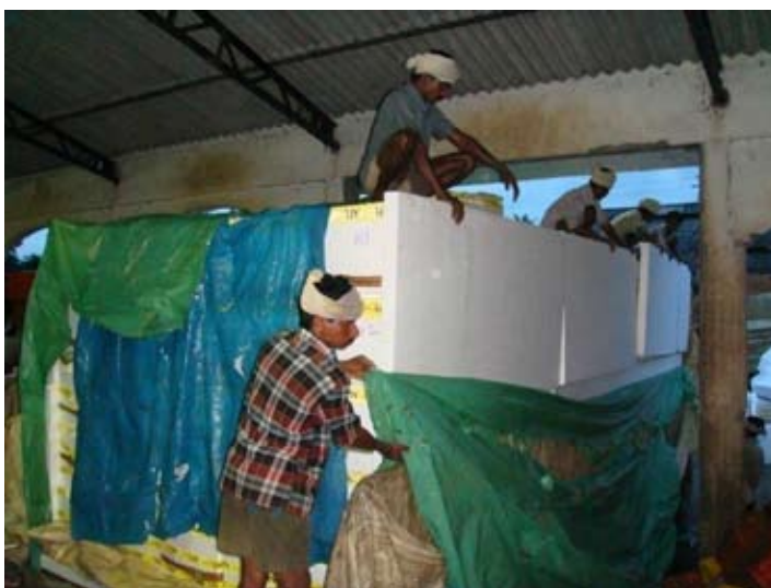
Truck loaded with fish kept in thermacol boxes are insulated with thermacol pads in a packing unit at Bhimavaram
